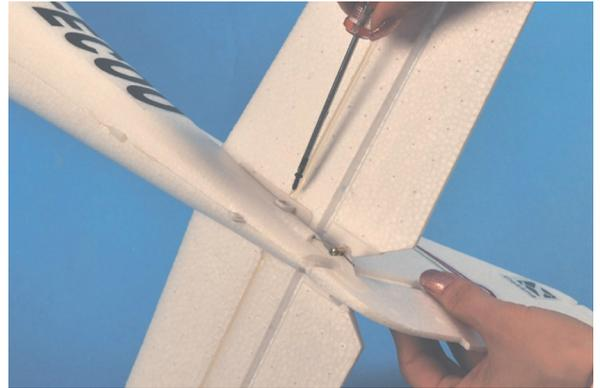
The horizontal stabilizer is secured with a locking screw.
