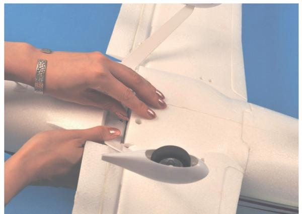
The tabs on the wing leading edge have to snap into the grooves.
